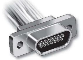
Micro-D Pre-Wired Pigtails-These connectors feature gold-plated TwistPin contacts and mil spec crimp termination. Specify nickel-plated shells or cadmium plated shells for best availability. 100% tested and backpotted, ready for use.
